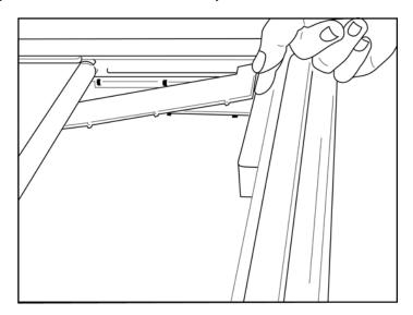
☐ The paper tray spacer should be parallel with the rear wall of the writer tray, as pictured below.
