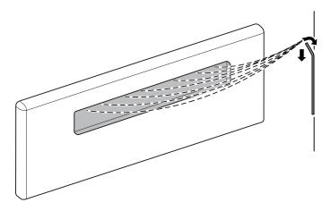
5. Secure the unit to the wall using the "A" screw.
