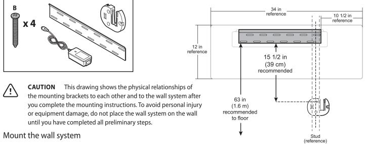
1. On the selected wall, find and mark the studs, and choose the system height and corresponding height for the mounting rail bracket.
